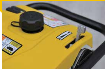
Throttle operation with integrated engine shutoff.
