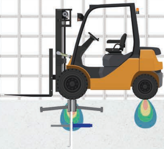
Load distribution at joint for S-Type
