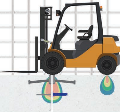
Load distribution at joint for straight type
